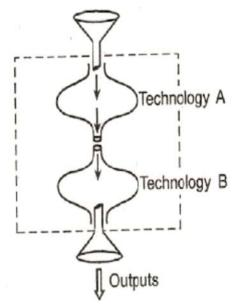
Fig. 5.1 shows a sequential hybrid system.
