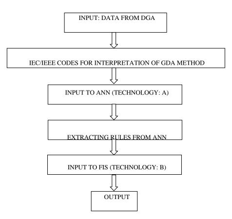
Fig. 5.2 Schema of proposed Diagnostic system
